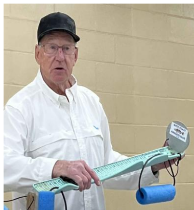
Bob created this unique fish measuring tool. He stills the fish with bungee cords head and tail.
